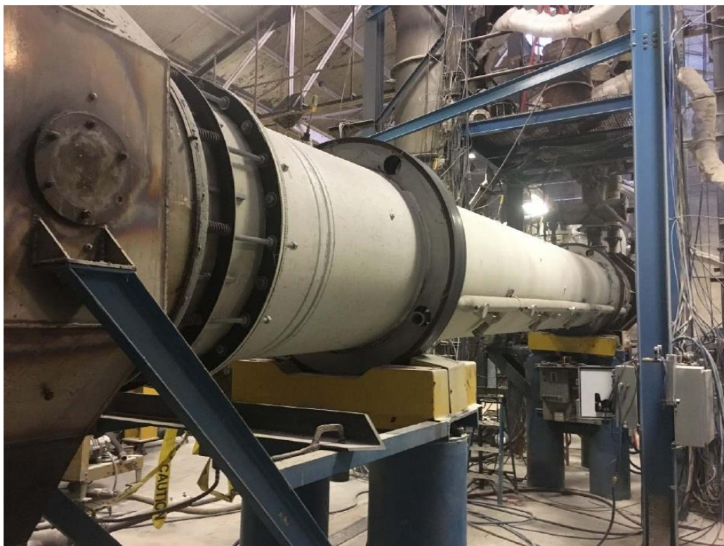
Figure 3: Pilot Rotary Kiln (9.8m long by 0.9m diameter) at FLSmidth Test Facility
